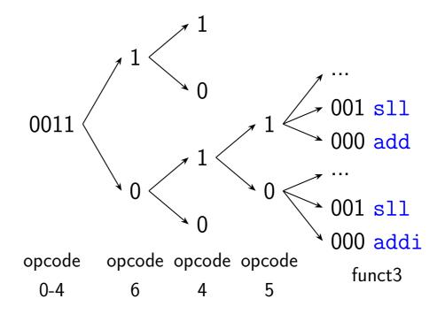
The opcode and function bits can be used to directly drive control lines (multiplexers, etc.)
